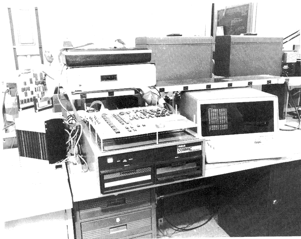
Fig. 9 - 16-bit bit-slice target system connected to development aids for software/hardware development and in-circuit emulation.
